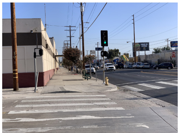
An example of a continental crosswalk.
